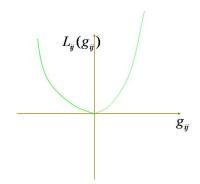
Figure 3: Characteristic dependence of power loss  $L_{ij}$  on the power flow  $g_{ij}$
