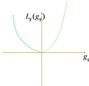
Figure 3: Characteristic dependence of power loss  $L_{ij}$  on the power flow  $g_{ij}$
